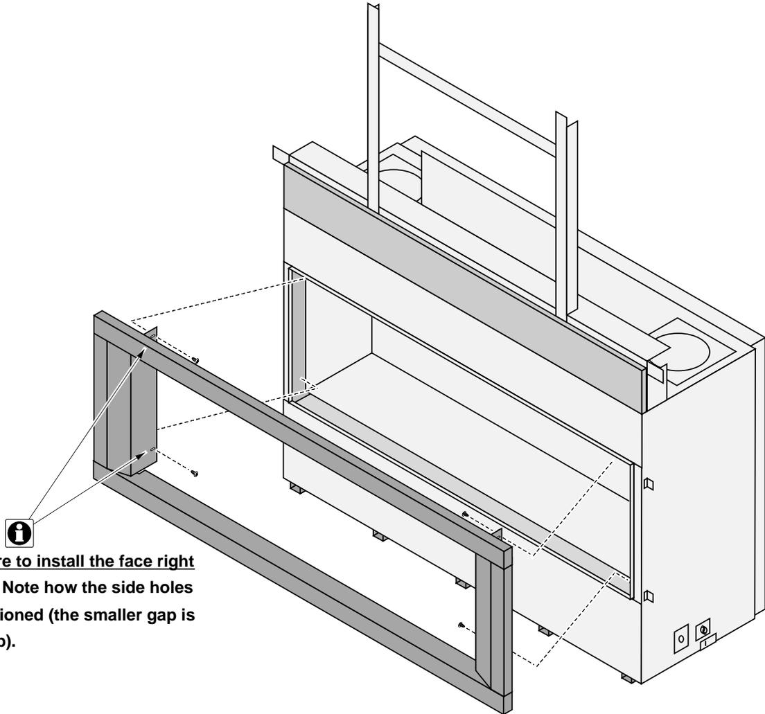
**Make sure to install the face right side up. Note how the side holes are positioned (the smaller gap is to the top).**
