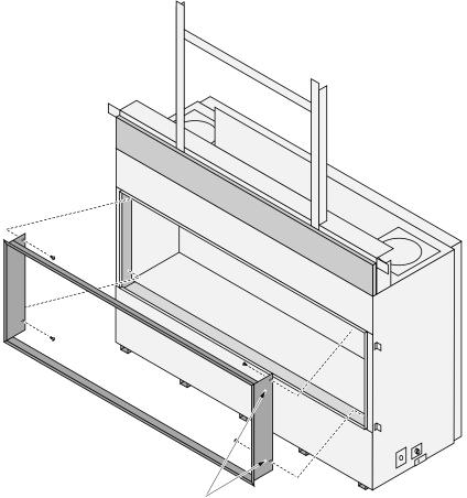
Make sure to install the trim right side up. Note how the side holes are positioned (the smaller gap is to the top).
