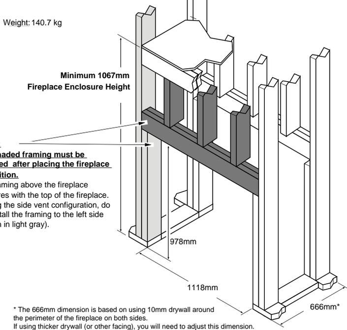
\* The 666mm dimension is based on using 10mm drywall around the perimeter of the fireplace on both sides. If using thicker drywall (or other facing), you will need to adjust this dimension.
