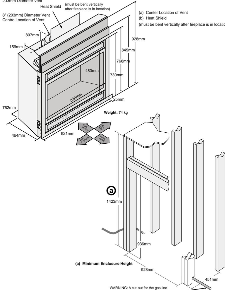
WARNING: A cut-out for the gas line may be required on the framing. See the dimensions under "Gas Line Connection" for details.
