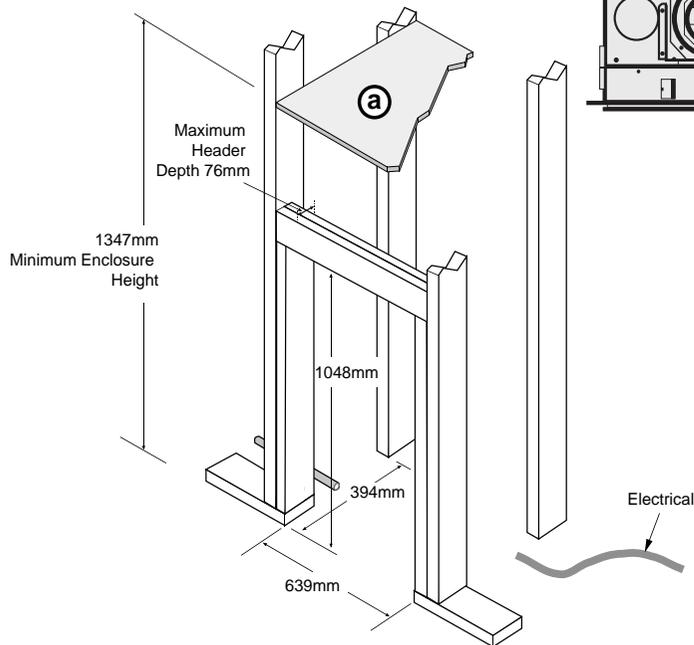
**a** The fireplace enclosure must be a minimum of 1347mm tall. Do not build into the fireplace enclosure
