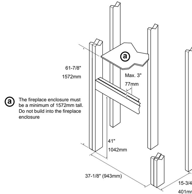
**a** The fireplace enclosure must be a minimum of 1572mm tall. Do not build into the fireplace enclosure
