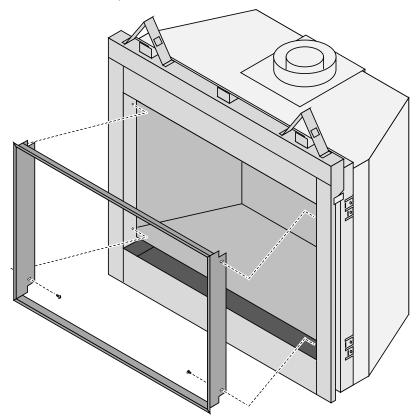
When tightening the screws, push the trim against the facing to ensure a seamless fit.
