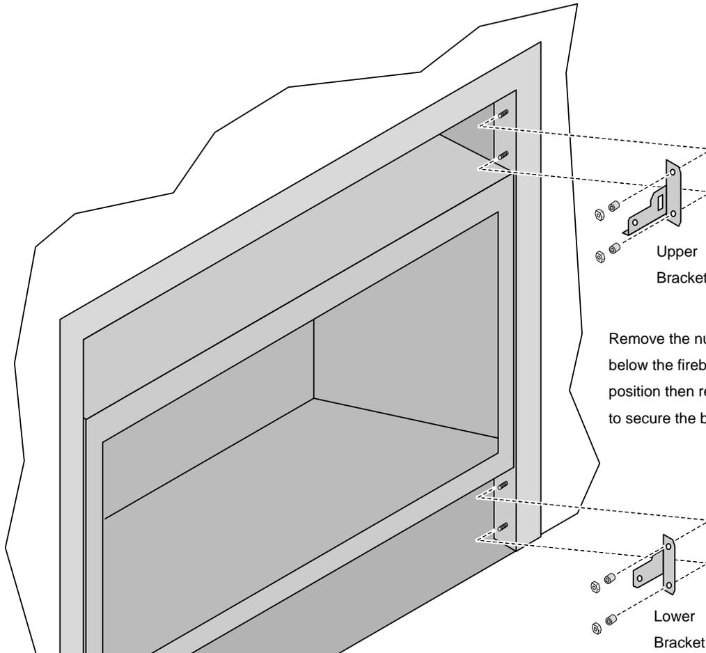
Remove the nuts and bushings above and below the firebox. Place the brackets into position then replace the bushings and nuts to secure the brackets in place.
