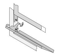
Bend the tab outward on both sides. This is the end-stop for the lower grill, it allows the grill to swing forward.
