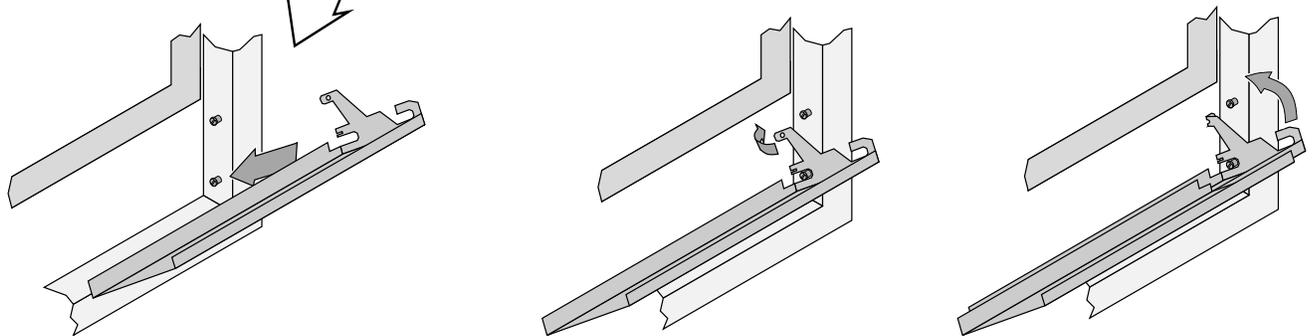
Hold the grill at an angle and insert the lower slot over the bushing on the fireplace (both sides). You may need to press on the grill to get the tab over the bushing (this prevents the grill from accidentally falling off).
