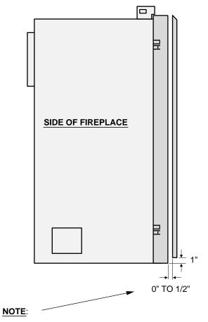
This face has an adjustable bracket that allows for different facing depths to be tucked under the face.
