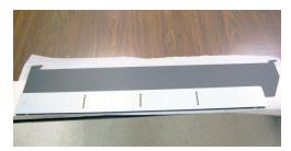
2. We recommend clamping the template and mounting brackets together to ensure proper alignment.
