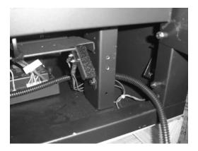
Press the wire hanger clips into the switch box (see the two white arrows in the picture below). Attach the switch box to the right side support leg with two of the included #8 Phillips screws (see circle in picture below).
