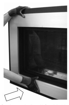
6 Check the corners of the face opening to make sure the face is properly aligned left to right (photo below). The face may be adjusted slightly to ensure correct alignment.
