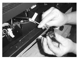
Pull the knob off the accent light rheostat. Unscrew the rheostat nut to remove the rheostat from the control panel. Disconnect the two wires leading to this rheostat.
