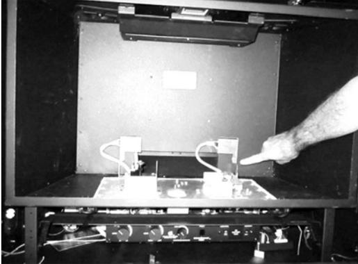
Figure 1: Accent light bracket screws location
