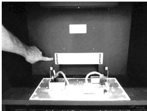
Figure 4: Intake restrictor installed, showing location of screws
