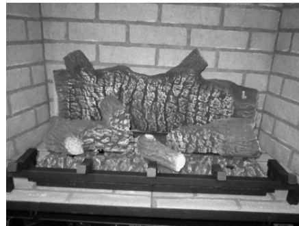
Figure 16: Center Ember Chunk Installed
