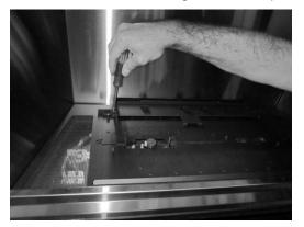
5. Install the front stone grid onto the burner.
