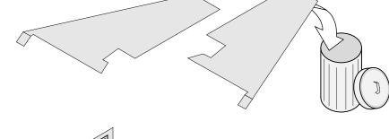
Remove the exhaust restrictor from the firebox ceiling (it is replaced after firebacks are installed).
