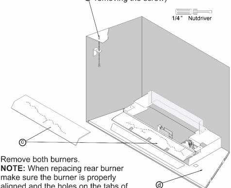
**NOTE:** When repacing rear burner make sure the burner is properly aligned and the holes on the tabs of the burner insert over the pins on the burner stand.
