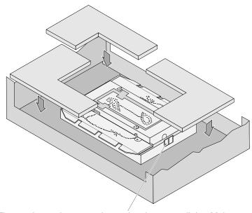
NOTE: These tabs are bent out when using the accent light. Make sure to carefully bend them flush if the accent light was previously installed (then reposition them after firebacks are installed).
