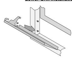
Hold the grill at an angle and insert the lower slot over the bushing on the fireplace (both sides). You may need press on the grill to get the tab over the bushing (this prevents the grill from accidentally falling off).
