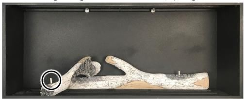
• Install Log #6 as shown below. The wide end of the log faces the front of the fireplace. The Log Locating pin on left of Log #5 insert into the hole on the bottom of log #6. Log #6 spans the burner.
