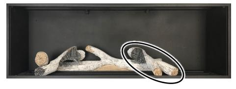
• Install Log #9 as shown below. There are no locating pins for this log. This log does not span the burner. The left end of the log rests on the right end of Log #2 and the right end rests on the rear portion of the media tray. Make sure the log does not cause any flame impingement.
