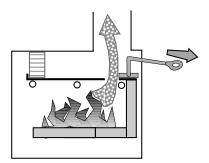
Bypass Pushed In Used for normal operation
