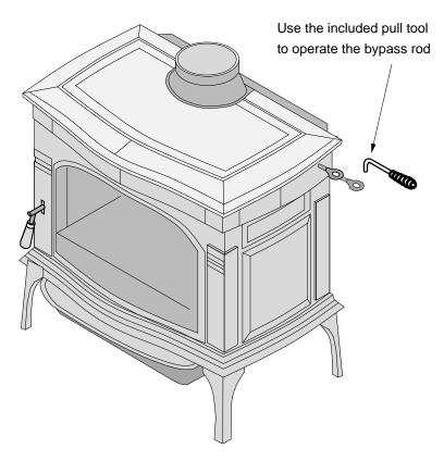
Bypass Pulled Out Used for starting and re-loading
