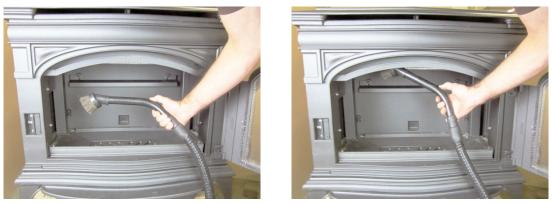
2. Carefully place the brush surface of the nozzle over the post combustor openings and remove any ash or debris. Take care to prevent damage to the post combustor (the surface is fragile).
