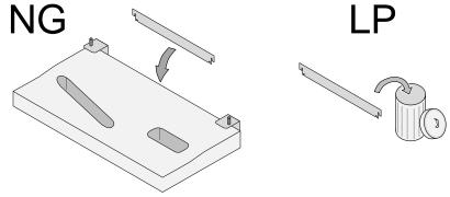
Install the burner. Install the side ember trays.
