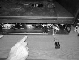
The last step is to verify the switch bracket properly contacts the micro switch on the insert: NOTE: This step is best done with the glass removed.
