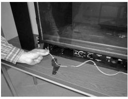
Insert the on/off wires through the switch bracket and attach to the on/off switch.
