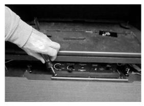
The switch bracket attaches to the Shadowbox face. Remove the two lower inside nuts (see photos below). Place the switch bracket over the studs and secure using the nuts removed earlier.
