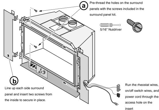
DVS and DVL Insert EF II – Top Panel and Trim Installation
