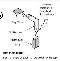
and side trim piece. Align the trim to form a precise corner, then tighten the two set screws with a small standard screwdriver. Slide the trim over the panels. Place the spring clips behind the panels at the locations shown. This keeps the trim tight against the panel.
