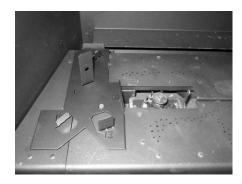
6. Place the rear stone grid on the burner as shown below.
