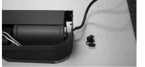
2 Disconnect the power cord from the blower. Route the power cord out of the blower housing and discard.
