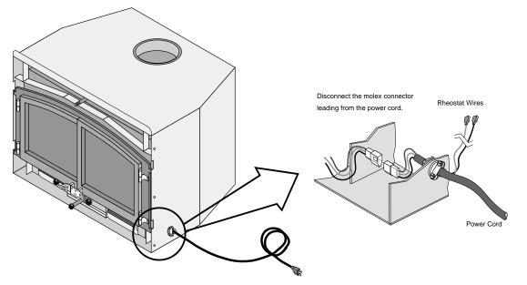
2 Remove the power cord as shown below. Tighten the strain relief on the two wires leading to the rheostat.
