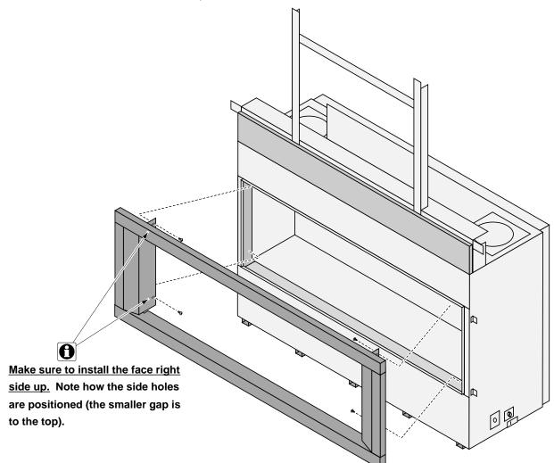
When tightening the screws, push the face against the facing to ensure a seamless fit.
