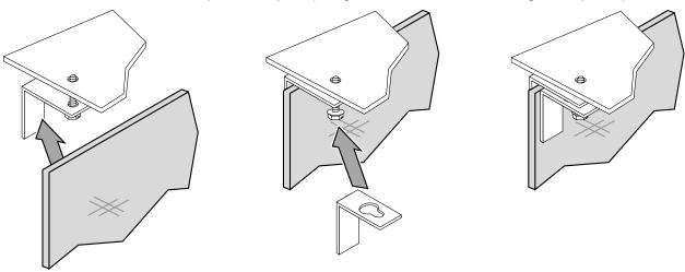
8 Install the two side "L" spacers included with this kit using the screws removed in step 2 (1/4" nutdriver). Leave the screws loose, they will be tightend in a later step.
