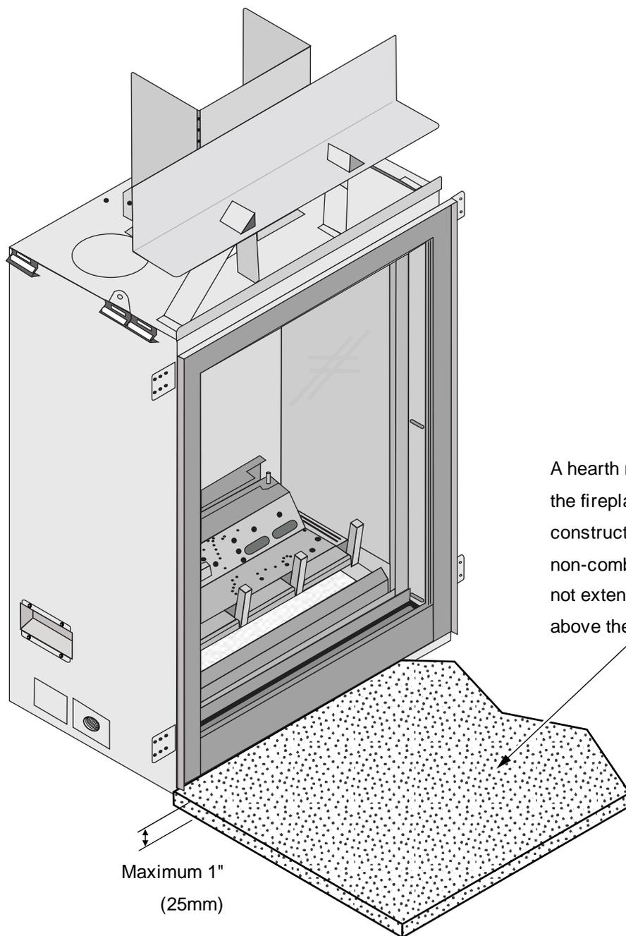
A hearth may be installed in front of the fireplace. The hearth can be constructed of combustible or non-combustible material and must not extend more than 1" (25mm) above the base of the fireplace.
