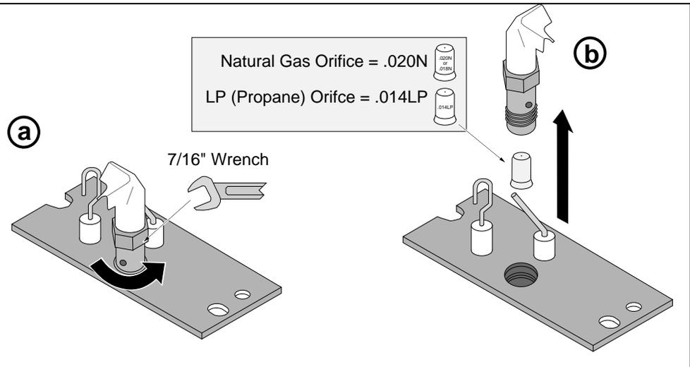
6. Remove the regulator from the front of the gas control valve. There is a knob extension on the regulator knob that will need to be moved to the new regulator. To remove the extension pull toward you. Replace with the propane regulator, using the new gasket and screws included with the regulator. Re-install the knob extension onto the LP regulator knob. The knob extension is directional so you may need to turn it until it lines up properly with the regulator knob and can be pushed into place.
