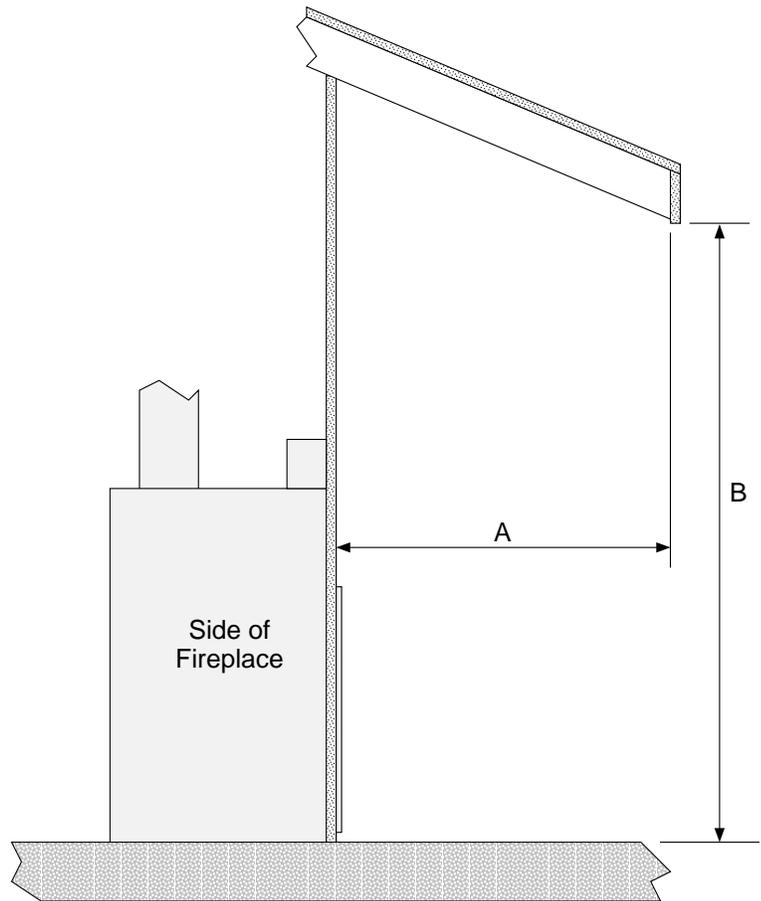
The overhang (A) must extend at least 1/2 the roofline height (B). Height is measured from the base of the fireplace.
