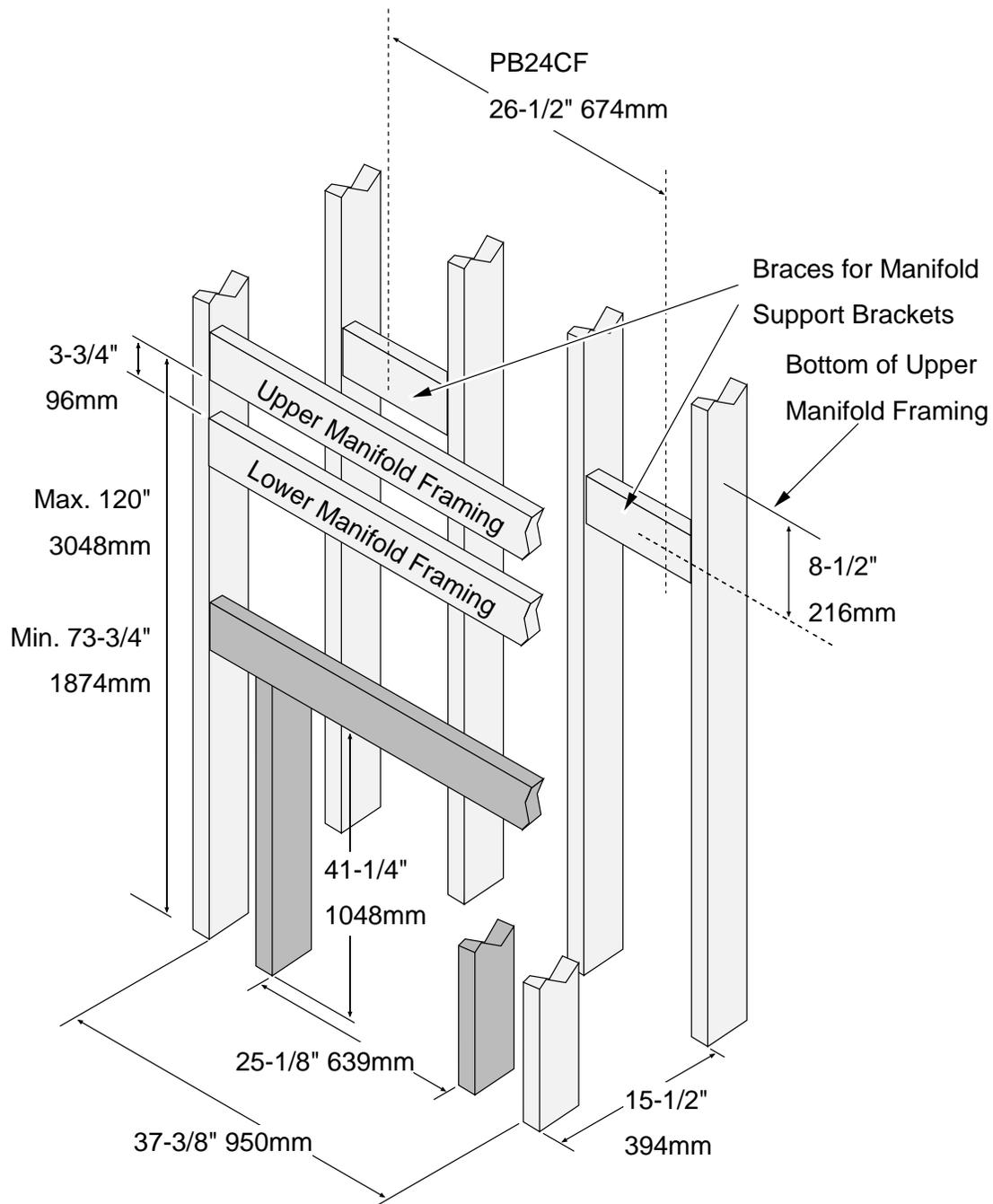
**NOTE:** The dark-shaded framing is typically installed after the manifold is installed. It is used to secure the nailing brackets on the fireplace to the framing. It also provides support for the facing above the fireplace. This framing is not required in some cases (you may use other methods to secure the nailing brackets and facing).
