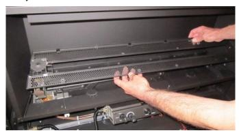
• Locate the burned out bulb and remove it from the socket by pulling the bulb directly away from socket (do not twist).
