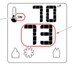
This is the target temperature on the read-out. Use the up or down buttons to adjust the target temperature.
