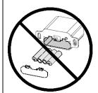
The remote control system requires the batteries and battery cover to remain in place at all times. Once the batteries or cover are removed, the system may restart in standing pilot mode. If this occurs when the heater is in Remote Mode, you will not be able to turn off the heater manually from the battery box.
