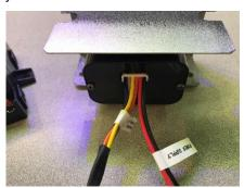
8. Attach the remaining connector with the red and black wires to the wire harness where the battery box was disconnected from in step 4.
