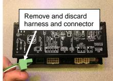
4. Install the system jumper into the same location on the board that you removed the green connector in the previous step.
