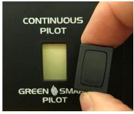
3. Follow the green and white wires to where they attach to the control module. Disconnect the green, plastic connector from the control module by lifting straight up (location is marked X4 on the module). Remove the connector and wires from the unit and discard. Install the switch blank into the empty mounting hole of the switch that was removed.
