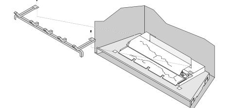
3 Remove the grate and set aside for reinstallation.
