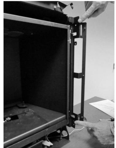
5. Replace the screw removed in step 2.
