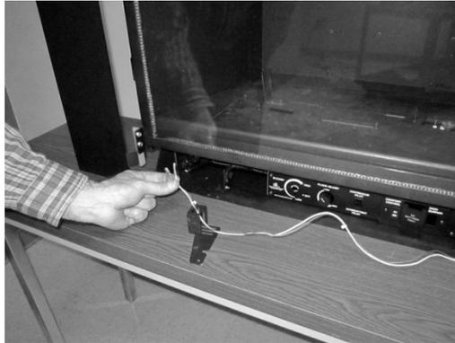
Insert the on/off wires through the switch bracket and attach to the on/off switch.
