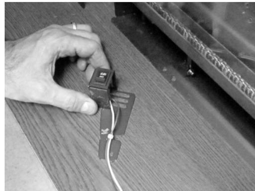
Insert the switch into the bracket, and then attach the bracket to the insert using an included screw. Secure the wires to the insert, making sure they do not contact any hot or moving components (use lock-ties if necessary). (NOTE: The 1-piece panels already have this screw installed.)
