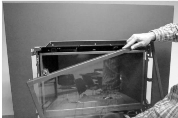
7. Attach the face to the hinge bracket with the included nuts.
