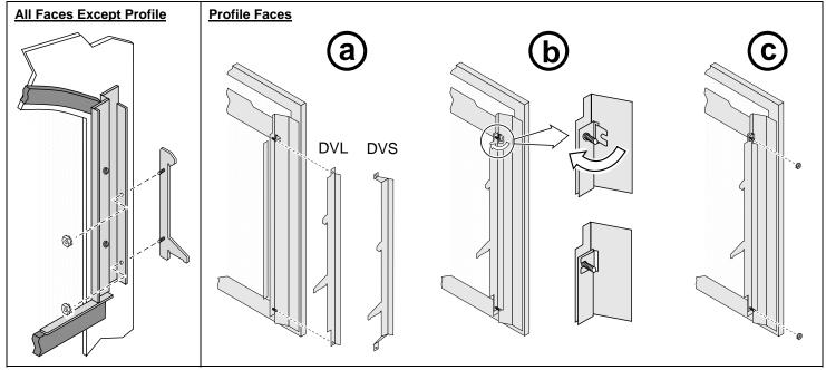
3 The face mounts to the insert as shown in the illustration to the right.
