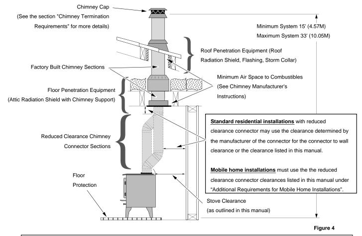
**Drafting Performance** This appliance relies upon natural draft to operate. External forces, such as wind, barometric pressure, topography, or factors of the home (negative pressure from exhaust fans, chimneys, air infiltration, etc.), may adversely affect draft. Travis Industries cannot be responsible for external forces leading to less than optimal performance.
