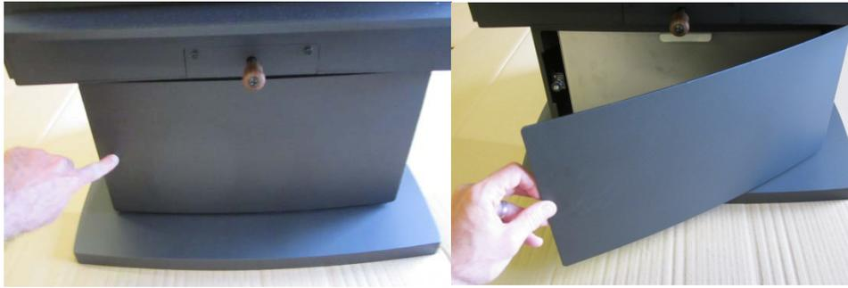
Slide the ashpan out and use the included handle and lifting rod to remove the ashpan.
