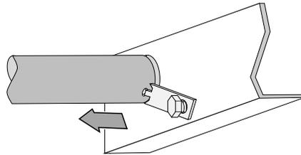
With the bolt loosened the air tube can be slid out of the air channel.
