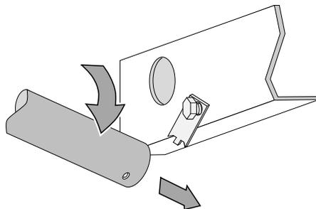
Pivot the air tube downwards and slide it out of the air channel on the opposite side.
