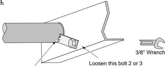
Note how the center of the air tube pin inserts into a hole on the air tube. Loosen this bolt 2 or 3 turns (do not remove).
