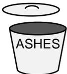
Ashes should be placed in a metal container with a tight fitting lid. The closed container of ashes should be placed on a noncombustible floor or on the ground, away from all combustible materials, pending final disposal. If the ashes are disposed of by burial in soil or otherwise locally dispersed, they should be retained in the closed container until all cinders have thoroughly cooled.
