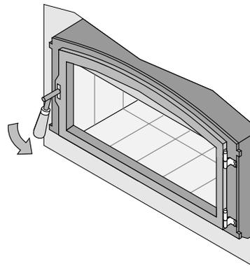
Rotate the handle down to secure the door.
