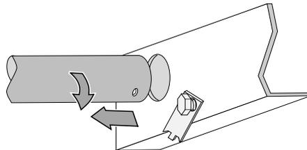
The pin will then disengage from the air tube (you may wish to rotate the tube slightly).
