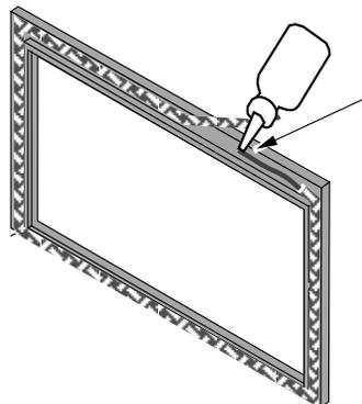
Use RTV high temperature silicone to adhere any loose gasket.
