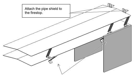
Secure the pipe shield to the vent with the included screws (use the 6 brackets). Make sure the pipe is placed so it protrudes over the elbow as shown below.
