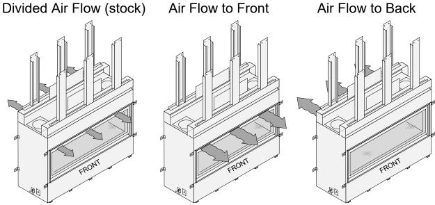
To adjust the air deflector, remove the glass frame and locate the two 3/4" holes in the firebox ceiling. Use a 7/16" nutdriver (or socket wrench) to adjust the deflector.
