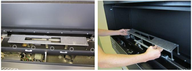
5. Remove and discard the NG (stock) manifold cover and orifice gasket (1/4" nutdriver). Install the LP manifold cover included in the owner's pack.
