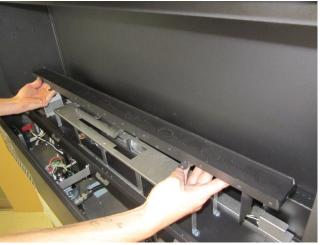
4. Remove the burner support as shown below. It is held in place with 10 screws (1/4" nutdriver).
