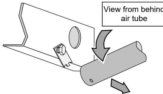
Pivot the air tube downwards and slide it out of the air channel on the opposite side.
