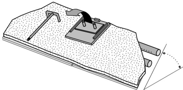
9. Lift the bypass damper off the slide plate and remove it from the inbuilt (see below).
