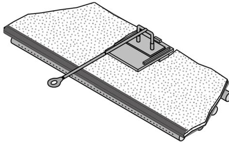
2. Unscrew and remove the bypass damper rod and ring from the damper yoke.
