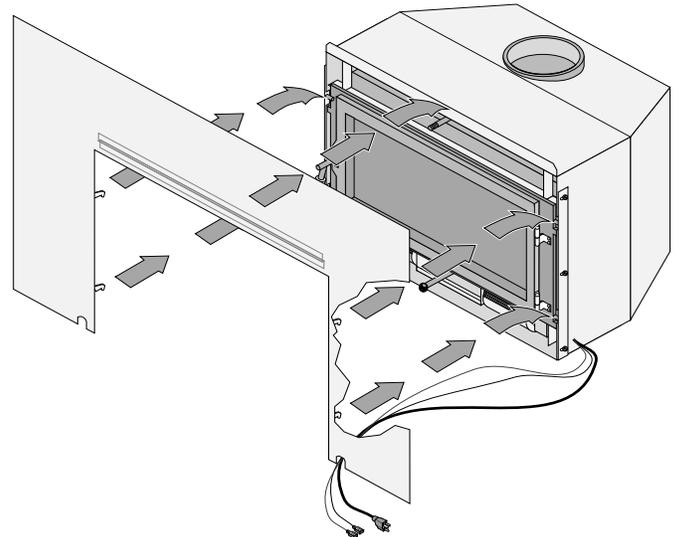
**HINT:** When installing the panel, route the wires through the notch on the bottom of the panel (either side).
