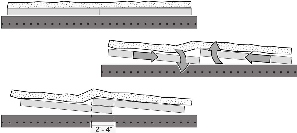
12. With the baffle board overlapping each other, both baffle board pieces and the blanket should now fit through the inbuilt door opening.
