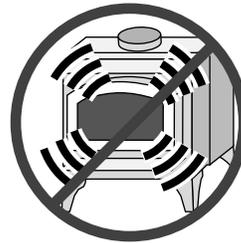
Over-firing the appliance may cause a house fire. If a unit or chimney connector glows, you are over-firing.
