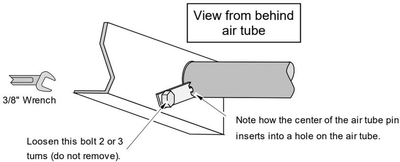
Note how the center of the air tube pin inserts into a hole on the air tube.
