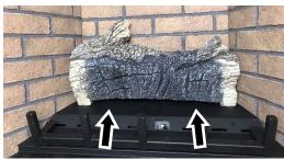
Place the left log on the lower front portion of the burner. The notch on the bottom left of the log rests on the grate. Push the log backwards until it is in contact with the sloped area between the front and rear burner.
