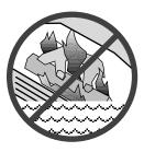
Do not operate if any portion of the heater was submerged in water or if any corrosion occurs. Immediately call a qualified service technician to inspect the appliance and to replace any part of the control system and any gas control that has been under water.
