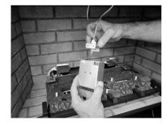
5. Loosen the two screws nearest the bulb to disengage the bulb from the holder. Remove the bulb from the holder. Replace the bulb, making sure not to touch the bulb with your fingers (grasp the bulb with the bulb packaging or a paper towel). Tighten the screws until the bulb is secure (do not overtighten, this may damage the electrical contacts on the bulb).
