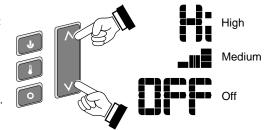
**HINT**: If you wish to leave the accent light on while turning the burner off, adjust the Flame Height to "OFF" (see above).
