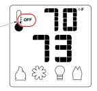
■ <u>SMART THERMOSTAT</u> – While in smart thermostat, the transmitter will control the burner to achieve the target temperature (see below). Flame height will be adjusted up or down to allow operation without turning the burner on and off (also called "smart modulation"). To adjust the target temperature, press the UP and DOWN buttons until a suitable temperature is achieved.
