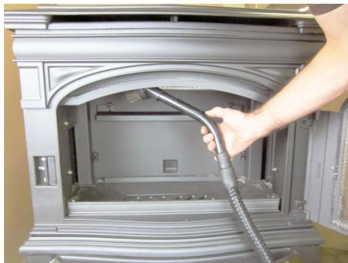
2. Carefully place the brush surface of the nozzle over the post combustor openings and remove any ash or debris. Take care to prevent damage to the post combustor (the surface is fragile).
