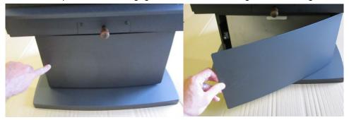
Slide the ashpan out and use the included handle and lifting rod to remove the ashpan.
