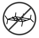
Do not use a grate or other device to elevate the fire off of the firebox floor. Burn the fire directly on the firebox floor.
