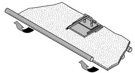
7. Lower the font edge of the baffle to gain access to the yoke and bypass components. Continue supporting the front edge of the baffle.
