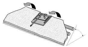
8. Lift the yoke out of the cups on the bypass damper and remove it from the inbuilt (see below).
