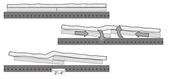
12. With the baffle board overlapping each other, both baffle board pieces and the blanket should now fit through the inbuilt door opening.
