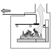
Bypass Pushed In Used for normal operation
