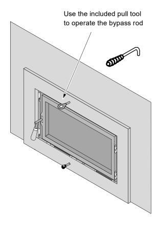
Bypass Pulled Out Used for starting and re-loadir
