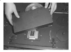
Remove the two screws securing the accent light assembly. Place the assembly upside down on the firebox top, making sure the wiring is not damaged or dislodged. When replacing, make sure the glass is aligned below the assembly.
