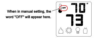
■ <u>SMART THERMOSTAT</u> – While in smart thermostat, the transmitter will control the burner to achieve the target temperature (see illustration below). Flame height will be adjusted up or down to allow operation without turning the burner on and off (also called "smart modulation"). To adjust the target temperature, press the UP and DOWN buttons until a suitable temperature is achieved.
