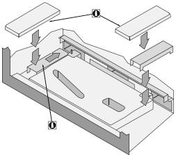
9 Place the two rivets into the burner holes shown below.
