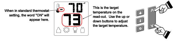
**NOTE:** If the transmitter batteries go dead while in thermostat setting (standard or smart), the appliance will shut off after approximately 24 hours.
