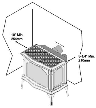
Rear vent installations may not use an elbow with a horizontal termination. We recommend using a top vent configuration if placed in a corner
