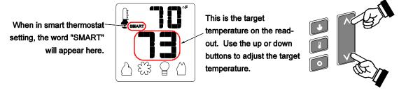
■ <u>STANDARD THERMOSTAT</u> - While in standard thermostat setting, the transmitter will turn the burner on and off to achieve the target temperature (see illustration below). To adjust the target temperature, press the up and down buttons until a suitable temperature is achieved.
