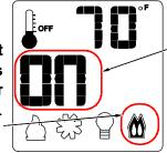
This is the comfort control read-out. Use the up button to turn on, down button to turn off (2 settings).
