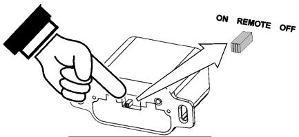
**NOTE**: When the battery holder switch is turned to ON or OFF, the mode settings (Flame Height, Comfort Control) will remain in the same state as before the switch was moved (i.e.: the IFC "remembers" the last setting). If you wish to adjust the mode settings use the transmitter mode button to adjust the settings (see "Mode Controls" on page 41). The thermostat and burner on/off operating functions will not work on the transmitter.
