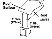
E Minimum 11" (279mm) clearance below unventilated soffits or roof surfaces
