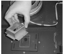
• Loosen the two set screws nearest the bulb to disengage the bulb from the holder. Remove the bulb from the holder. Replace the bulb, making sure not to touch the bulb with your fingers (grasp the bulb with the bulb packaging or a paper towel). Tighten the screws until the bulb is secure (do not overtighten, this may damage the electrical contacts on the bulb). When the bulb is inserted into the socket the two posts will be exposed approximately ¼" (6mm) – this is normal.
