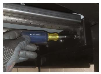
Push up on the baffle slightly and slide the front air tube to the left until the end is clear of the manifold. Lower the right end of the tube and maneuver left end of the tube out of the manifold on the left side of the firebox.
