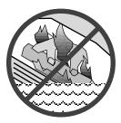
Do not operate if any portion of the heater was submerged in water or if any corrosion occurs. Immediately call a qualified service technician to inspect the appliance and to replace any part of the control system and any gas control that has been under water.
