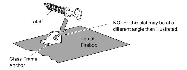
Note how the washer on the latch fits behind the flange on the glass frame anchor.
