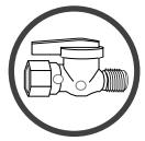
Instruct everyone in the house how to shut gas off to the appliance and at the gas main shutoff valve. The gas main shutoff valve is usually next to the gas meter or propane tank and requires a wrench to shut off.
