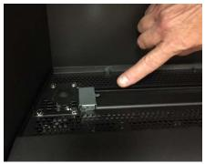
Spread an even layer of crushed glass over the media tray and burner. The glass must be only 1 layer thick on the burner but can be 2 layers thick on the media tray. **Make sure no glass is in the pilot area** indicated in the picture below.
