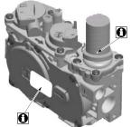
This heater is either approved for natural gas (NG) or for propane (LP). Burning the incorrect fuel will void the warranty and safety listing and may cause an extreme safety hazard. Direct questions about the type of fuel used to your dealer. Check for a label on the flame adjust knob on the gas control valve (this is the best place to check). You may also check for a label on the gas control valve body.
