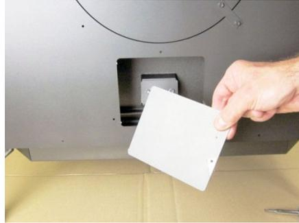
Remove the igniter cover plate and gasket. Retain the gasket and screws.
