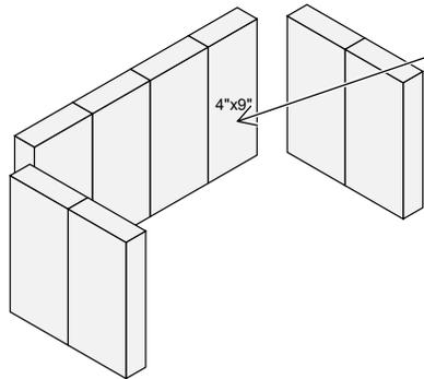
Remove this brick and replace it with the igniter firebrick. The Evergreen uses the brick included with the igniter, the Rockport uses the brick included with the stove.
