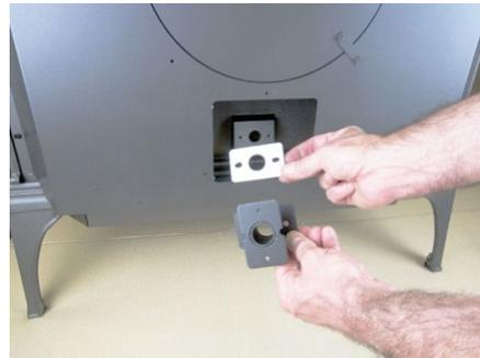
Install the igniter spacer using the screws and gasket removed in step 6. Make sure to use the screws that were removed with the gasket.
