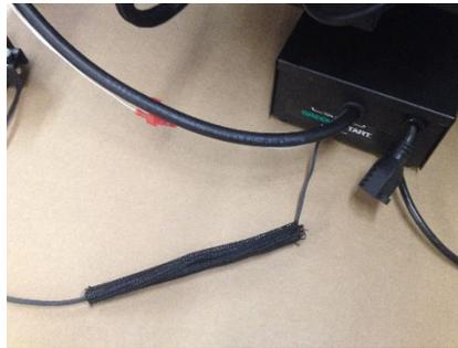
Place the longer piece of loom over the wires and tube leading to the igniter.
