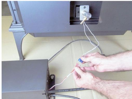
Attach the 1/4" tube to the nipple on the igniter.
