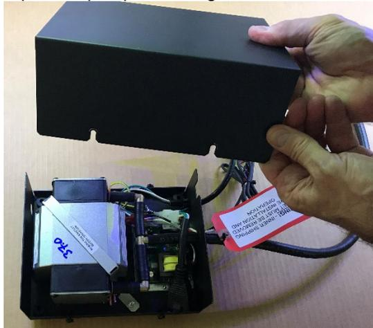
The outlet ships inside the housing. Route it through the slot and use the included strain-relief to hold the cable in place (see pictures below). Replace the cover.
