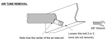
Note how the center of the air tube pin inserts into a hole on the air tube.
