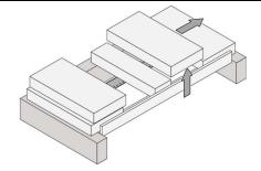
2. Push up on the center brick and rotate it slightly until you can lower it past the baffle support and remove it from the firebox.
