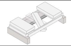
3. Rotate the bricks that were moved aside in step 1, lower them past the baffle support and remove them from the firebox.
