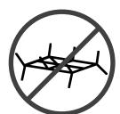
Do not use a grate or other device to elevate the fire off of the firebox floor. Burn the fire directly on the bricks.
