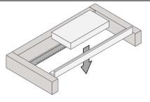
5. Push upward on the baffle support until it is above the side manifolds, rotate it slightly, and remove it from the firebox.
