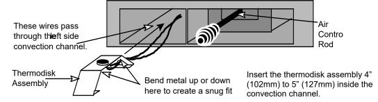
3 Install the wire clip following the directions below.
