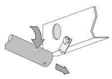
Pivot the air tube downwards and slide it out of the air channel on the opposite side.
