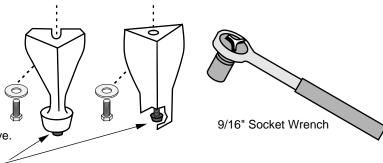
These rubber-tipped bolts are for leveling the stove. Make sure they contact the floor. Do not adjust with weight on the legs, the rubber tips may tear.
