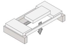
Push the two remaining bricks upward until you can rotate them. Lower them past the baffle support and remove them from the firebox.
