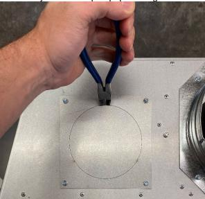
2. Grab on to the knockout with pliers and bend it back and forth until the remaining tabs break free. Discard the knock out plate.
