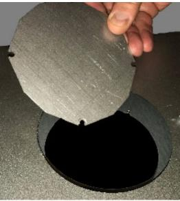
4. You will need to remove a third cover plate on each side. Remove the (2) 1/4" screws holding the cover plate in place. Reach in and remove the cover plate. You may discard this plate.
