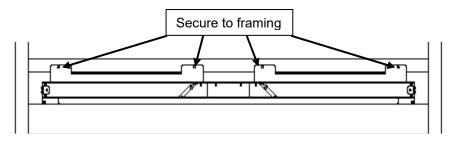
Re-attach the two rear mounting brackets (removed in step 6) to the bottom of the convection manifold. Leave the screws loose so the brackets can be positioned to the back of the chase. Secure the brackets to the chase using screws (not included). Tighten the screws securing the brackets to the manifold.
