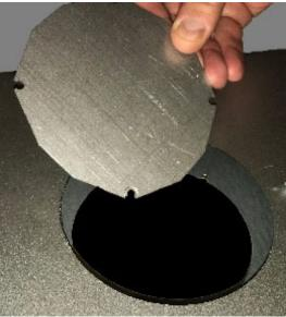
10. You will need to remove a third cover plate on each side. Remove the (2) 1/4" screws holding the cover plate in place. Reach in and remove the cover plate. You may discard this plate.
