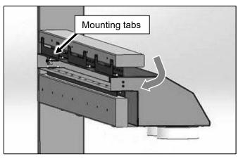
5. Secure the manifold to the upper framing using screws (not included).
