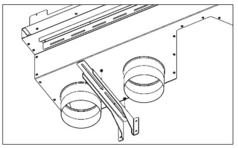
3. Determine the desired location of the bottom of the convection air outlet. Install a horizontal framing member at the desired height, parallel to the header. Install a second horizontal framing member 3-3/4" above the first. These two framing members will support the upper convection manifold in the following steps.
