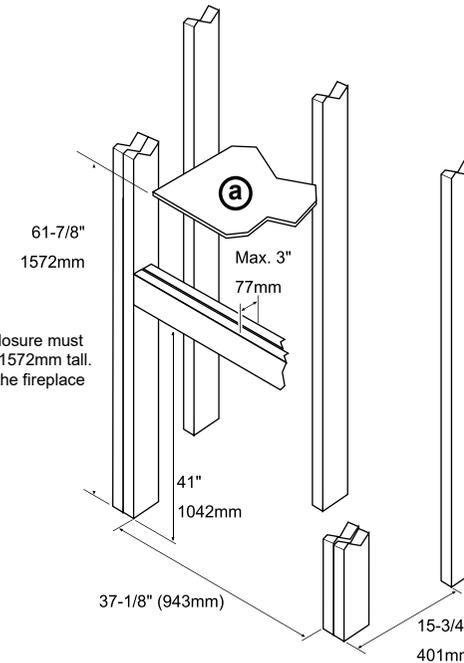
**a** The fireplace enclosure must be a minimum of 1572mm tall. Do not build into the fireplace enclosure
